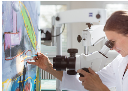
The mobile floor stand S covers a larger specimen space than any other stand available for Stemi 508. It is used to observe tall, heavy or irremovable specimens like car engines, large animals, living plants, sculptures or wall paintings
